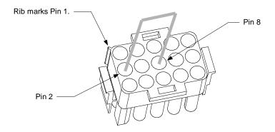
Insert a paper clip or wire into pins 8 and 2 of the 15-pin connector to ground pin 8.
